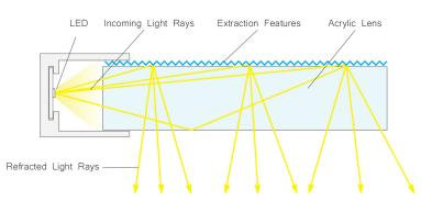
Edge lighting is a method of optical tranmission that Aron uses in many of our fixtures. Light coming from the LED shines into an acrylic lens. On the top side of the acrylic, surface bonded extraction features help to refract and spread light rays out of the arcylic to create various beam shapes.
