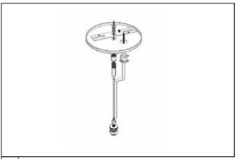
2 Attach canopy and suspension wire to preferred location. Hang suspension wire to specified length. Spacing of suspension wire should equal overall fixture length, minus 1"
