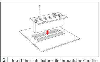
Insert the Light fixture tile through the Cap Tile.
