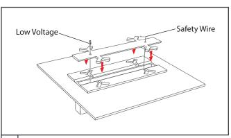
Feed low voltage wire and safety wire through the holes in the locking cap.
