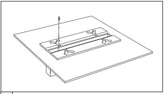
Push down the top flaps of the Light Fixture Tile against the adhesive on the Cap Tile.
