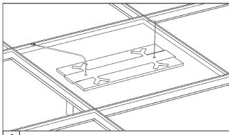
6 Install the Slot Light Fixture assembly into the T-Grid ceiling.
