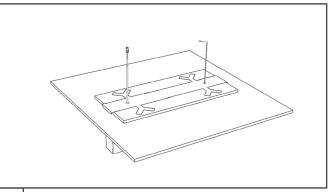
5 Push the Locking Cap Tile into the mating slots in the Light Fixture Tile.
