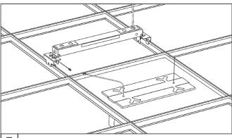
Install the Remote Driver on the T-Grid next to the Fixture. Attach the Power wire to the Driver and connect the fixture to the driver with the low voltage wires. Attach Safety Wire to structure.
