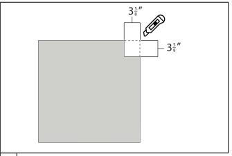
6 Cut 3 5/8" x 3 5/8" notch in ceiling tiles adjacent to fixture.
