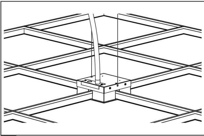
5 Complete electrical connection through fixture Access Plate.
