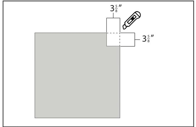
6 Cut 3 5/8" x 3 5/8" notch in ceiling tiles adjacent to fixture.
