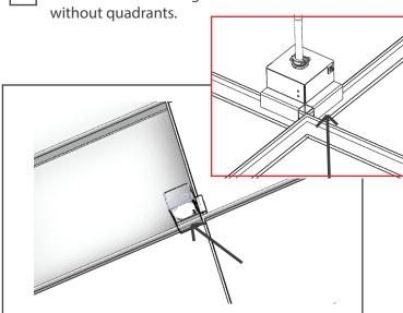
Lay fixture on the grid at the T-Bar intersection. Hooks on the side of the fixture sit on the TBar.
