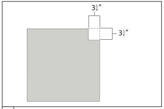
Cut 3 5/8" x 3 5/8" notch in ceiling tiles adjacent to fixture.
