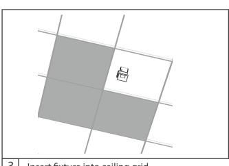
Insert fixture into ceiling grid.
