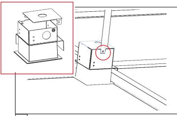
6 Unscrew hex heads located on the top of the driver box. Complete electrical connection through fixture Access Plate.
