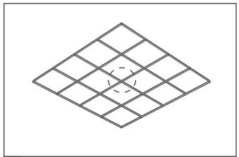
Prepare for QUAD installation by moving any tie wires away from intersection of grid where QUAD fixture will be installed.
