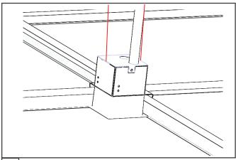
5 Tie fixture to deck using tie-up holes on the back of the fixture.
