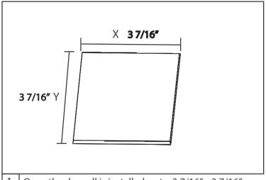
Once the drywall is installed, cut a 3 7/16" x 3 7/16" square for the fixture.
