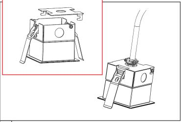
With the fixture still below the ceiling, complete all electrical wiring. Be sure that all sheet metal plates and boxes are secured.
