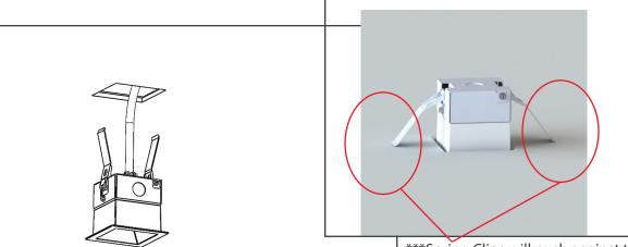
\*\*\*Spring Clips will push against the top of drywall to secure the fixture.
