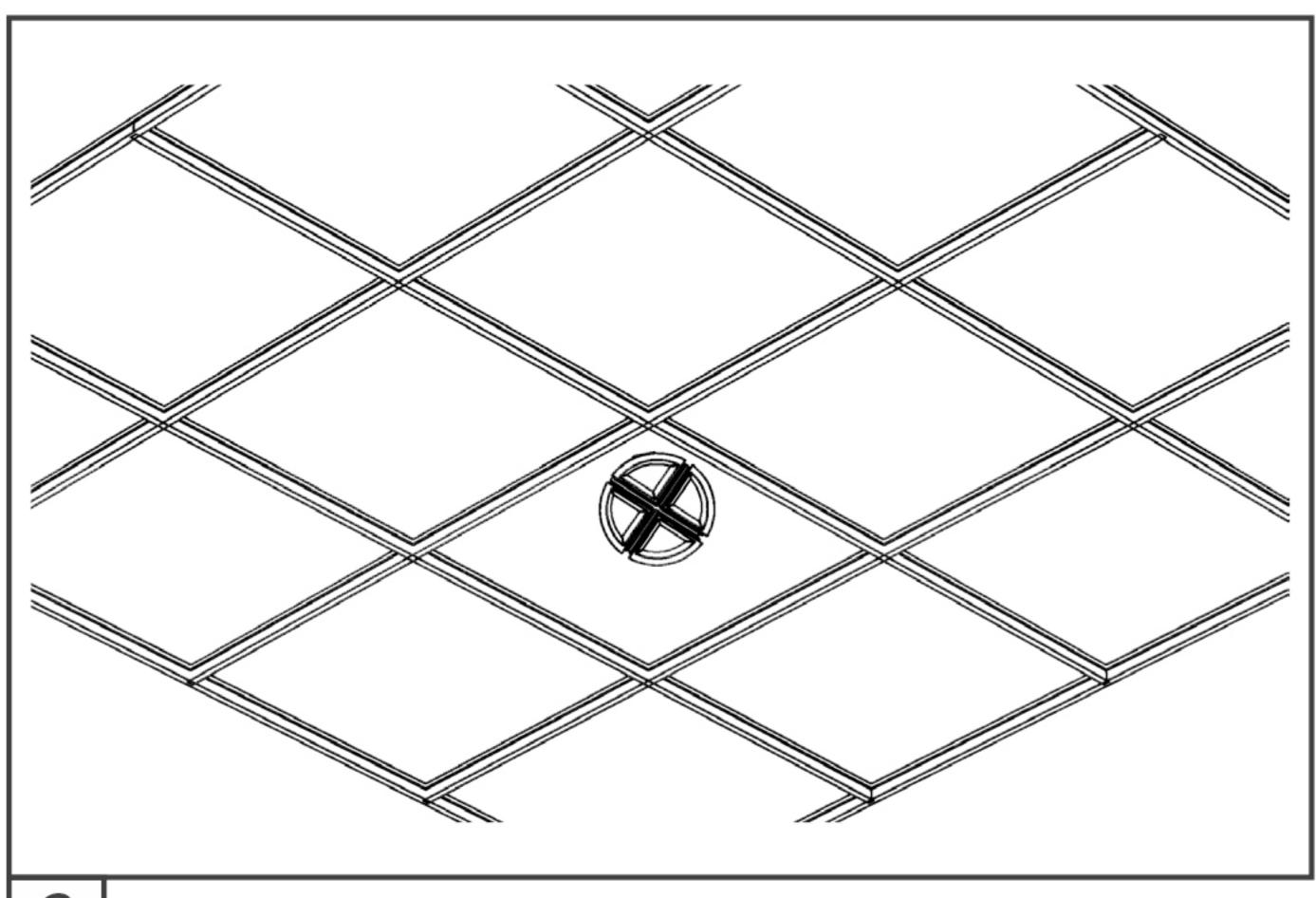
2 Insert fixture into ceiling grid.
