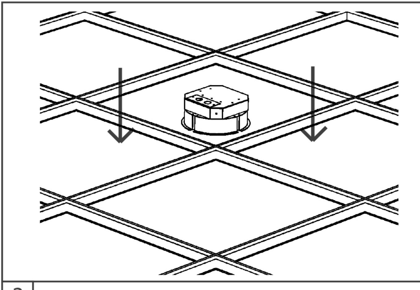
3 Lay fixture on the grid at the T-Bar intersection.
