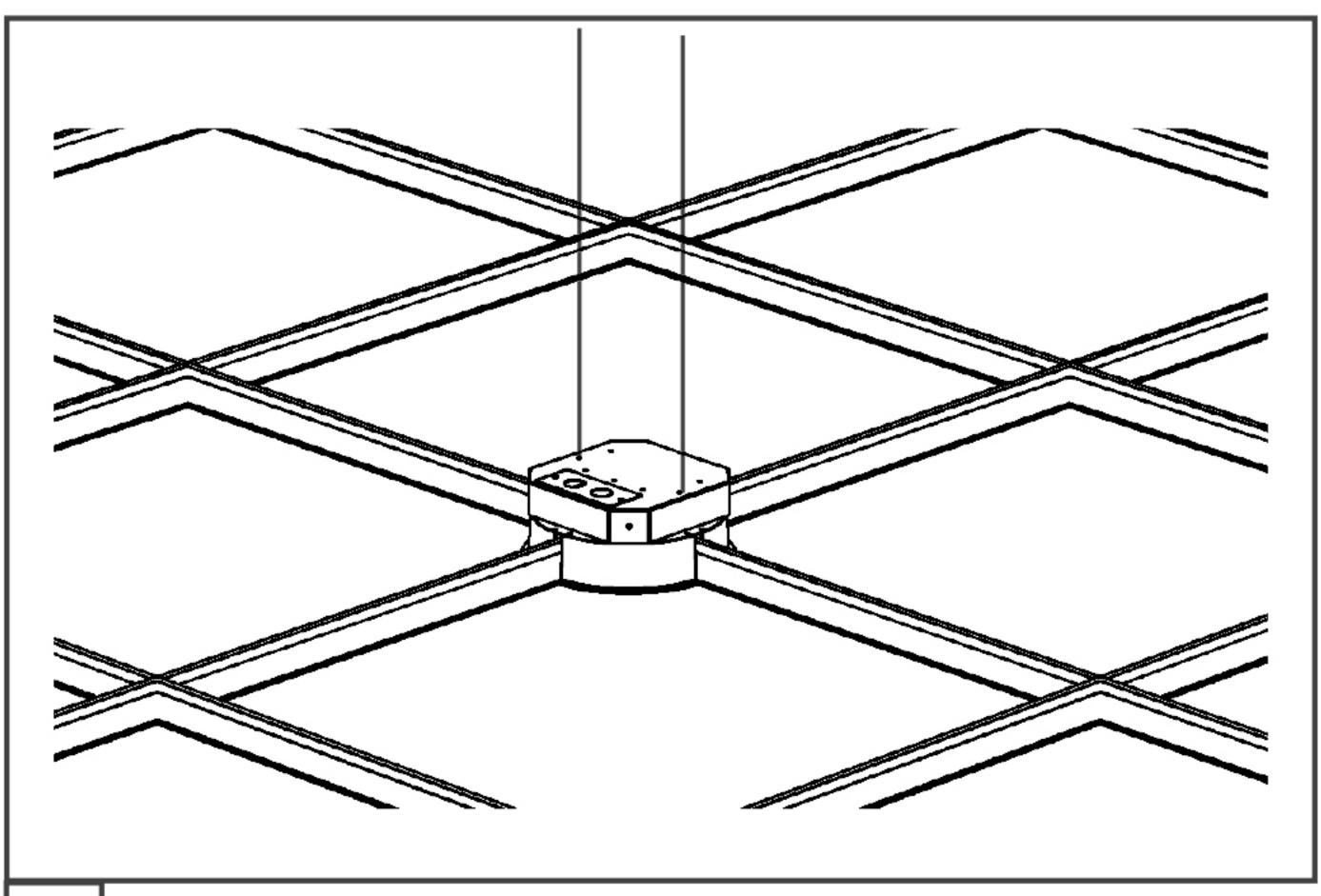
Tie fixture to deck using tie-up holes on the back of the fixture.
