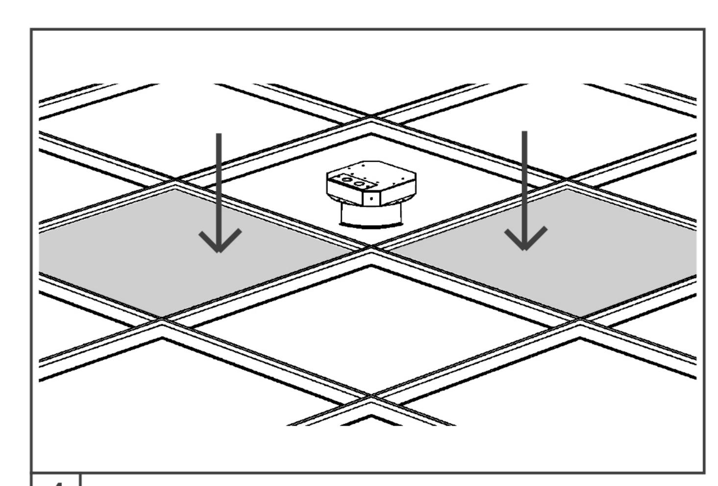
Lay fixture on the grid at the T-Bar intersection.
