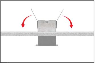
After installing the panel into the ceiling grid, insert the fixture through hole cutout and allow spring clips to gently grab the top of the ceiling tile. Ensure the flanges of the fixture are covering any ceiling tile cuts.
