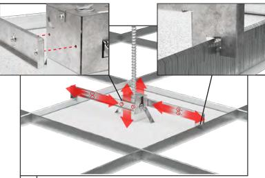
Install arm brackets by first sitting them on the t-bar and then screwing the bracket into the side of the fixture. See slot locations above to adjust height and length of arms.
