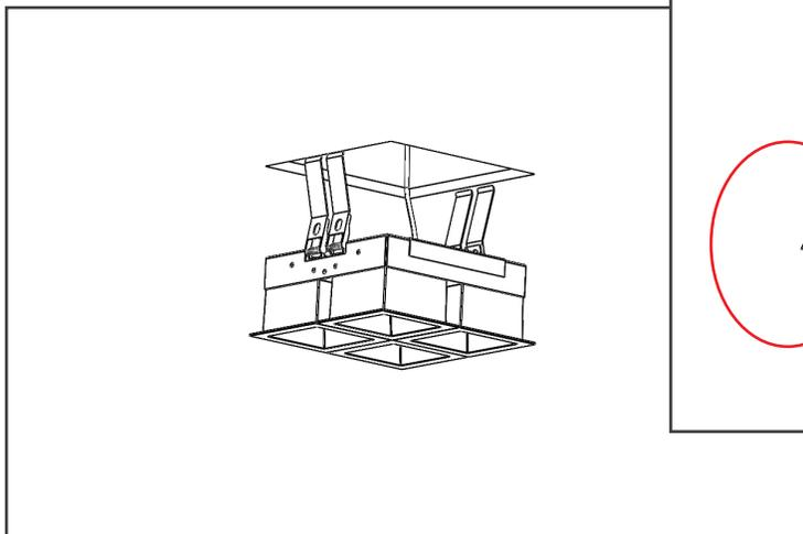
3 Bend Spring Clips upward and raise fixture into ceiling Hole.
