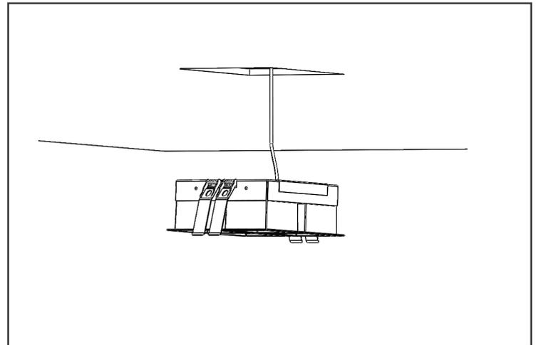
2 With the fixture still below the ceiling, complete all electrical wiring. Be sure that all sheet metal plates and boxes are secured.
