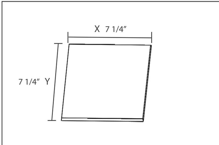
1 Once the drywall is installed, cut a 7 1/4" x 7 1/4" square for the fixture.
