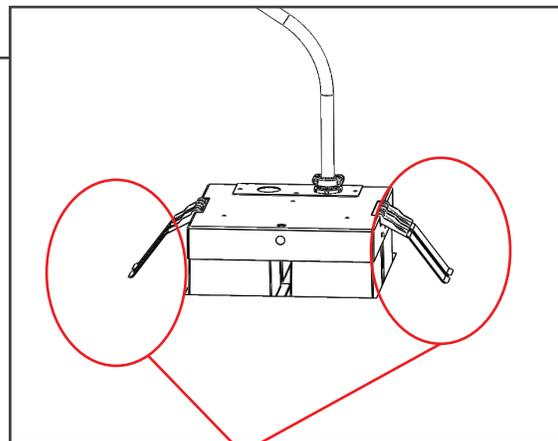
\*\*\*Spring Clips will push against the top of drywall to secure the fixture.
