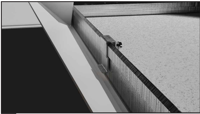
5 Install Seismic clips to left and right T Grid if needed.
