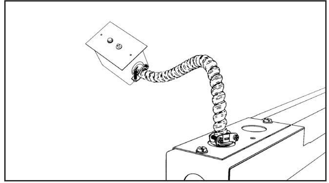
Install EM box using included plenum rated wire housing and connect to driver box housing through a knock out hole. Make necessary connections to driver.
