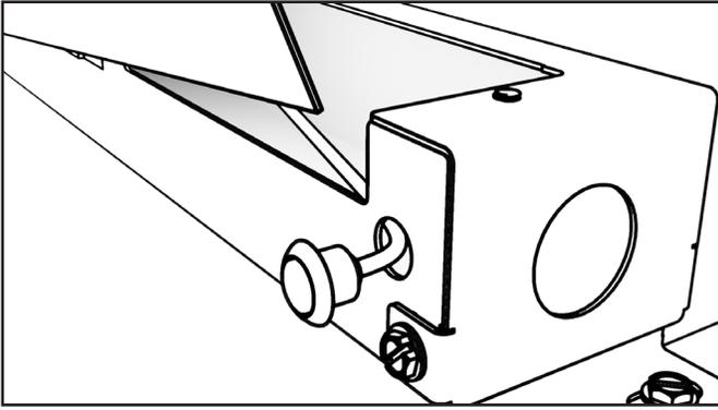
Install EM test button through side hole in driver box housing and secure using the included nut. Make necessary connections to driver.
