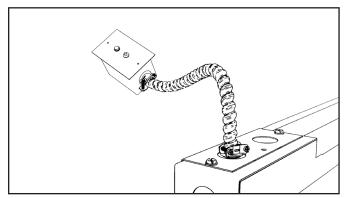
Install EM box using included plenum rated wire housing and connect to driver box housing through a knock out hole. Make necessary connections to driver.
