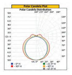
Length: 4ft Lumens/ft: 878.5 Total Lumens: 3513.8 Input Watts: 27.74 W
