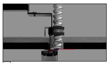
Pass low voltage conduit through notch in ceiling tile. Ensure metal conduit continues through ceiling tile and ends flush with bottom of tile.
