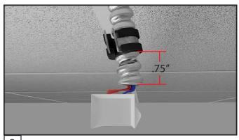
Attach loop clip to conduit .75" from the end.
