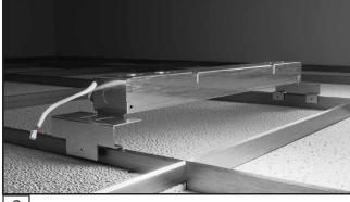
Install remote driver box within 5 feet of the wire passthrough hole by clipping it to the top of the T-grid. If surface mounting remote driver kit, remove T-Bar clips and mount to structure. Contact factory for longer power lead.
