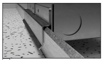
Install remote driver box within 5 feet of the wire passthrough hole by clipping it to the top of the T-grid.
