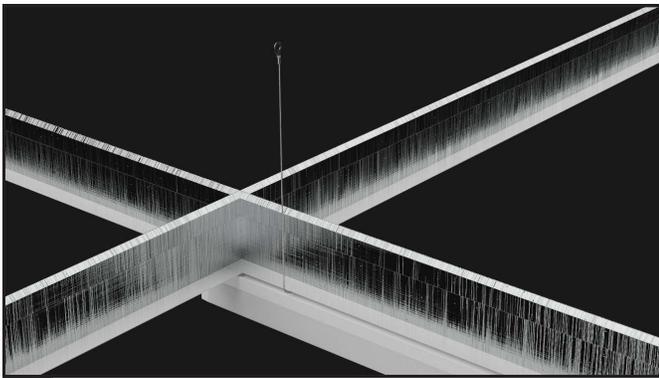
7 If required by code, attach safety wire to structure.
