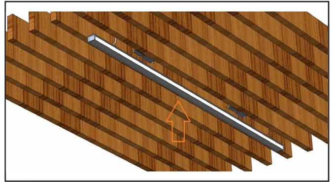
6 Once all the EZT T-Grid Brackets are in place prepare to install the fixtures to the magnets.
