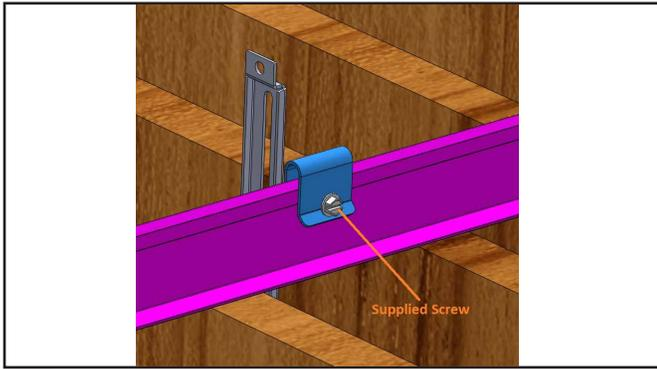
5 To keep the brackets from being removed from the T-Grid you can install the supplied screws into the top of the T-Grid Bracket to secure the brackets to the T-Grid.
