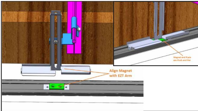
7 The magnets on the fixture should line up with the EZT T-Grid Brackets (a). Once the fixture is attached to the T-Grid Brackets ensure the magnets and Brackets are flush (b).
