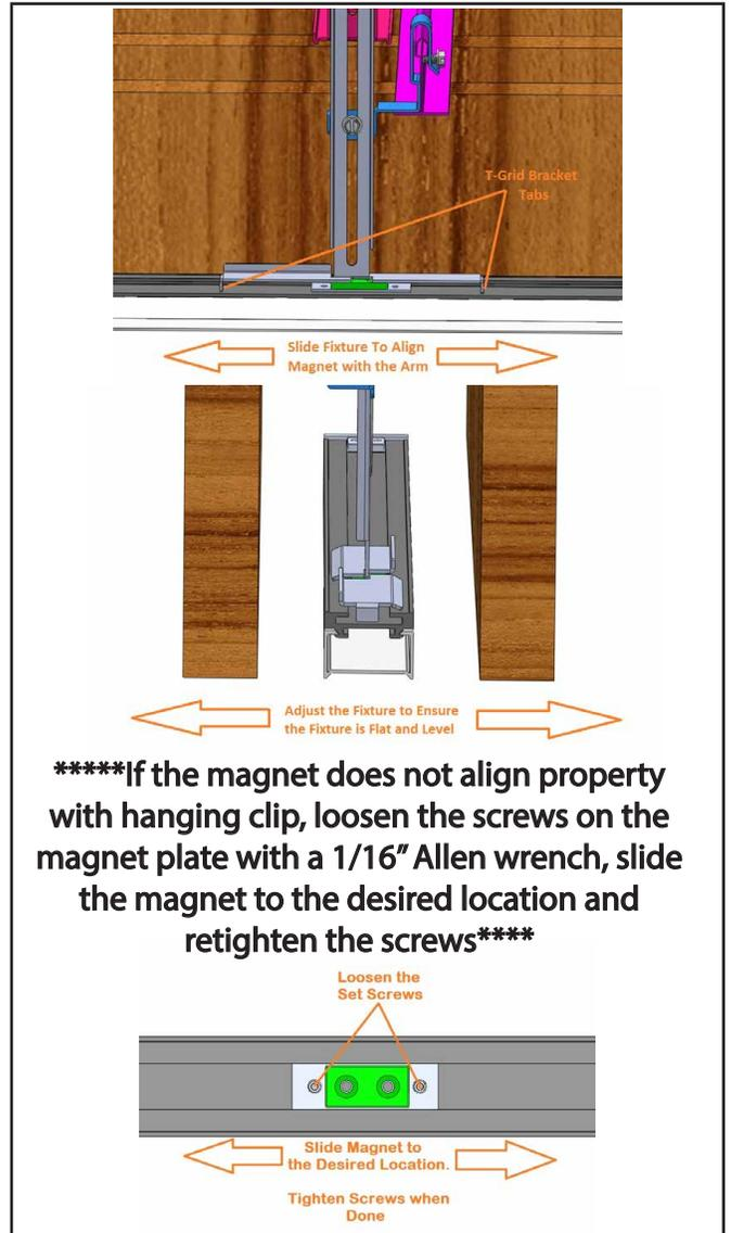
8 To adjust the alignment between the magnets and T-Grid Brackets move the fixture so the tabs on the T-Grid Bracket encompass the magnet and that the magnet and Bracket are flat and flush to one another.
