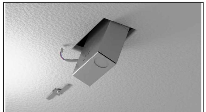
12 Install the driver housing to the selected surface.
