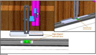
The magnets on the fixture should line up with the EZT T-Grid Brackets (a). Once the fixture is attached to the T-Grid Brackets ensure the magnets and Brackets are flush (b).
