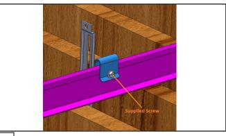
To keep the brackets from being removed from the T-Grid you can install the supplied screws into the top of the T-Grid Bracket to secure the brackets to the T-Grid.
