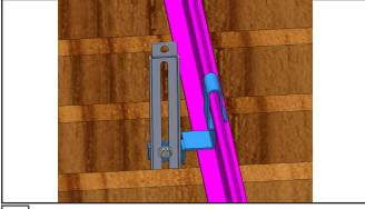
3 Install the EZTT-Grid bracket hanger onto the T-Grid.
