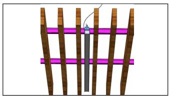
Make sure the fixture is centered between the wood slats.
