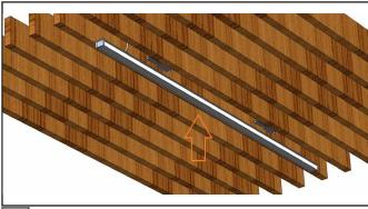
Once all the EZT T-Grid Brackets are in place prepare to install the fixtures to the magnets.
