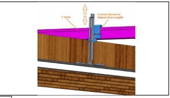
Adjust the length of the EZT Bracket Arm prior to installation to ensure the location of the light fixture will be flush with the bottom of the wood slats. Loosen the screw and adjust the arm length. Once you have identified the correct arm length, measure the length and adjust the rest of the arms for installation.
