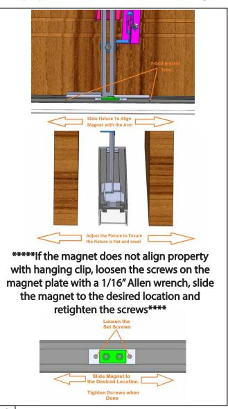
To adjust the alignment between the magnets and T-Grid Brackets move the fixture so the tabs on the T-Grid Bracket encompass the magnet and that the magnet and Bracket are flat and flush to one another.
