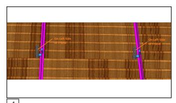
Install the additional Brackets along the same slot between the Wood Slats.
