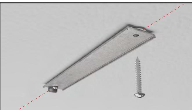
**3** Orient the Magnetic Drywall attachment plate to be inline with the fixture, then screw into Drywall Anchor. Tabs of plate should be facing downward.
