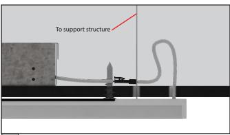
8 Feed safety wire through hole and attach to structure per code requirements.
