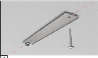
Orient the Magnetic Drywall attachment plate to be inline with the fixture, then screw into Drywall Anchor. Tabs of plate should be facing downward.
