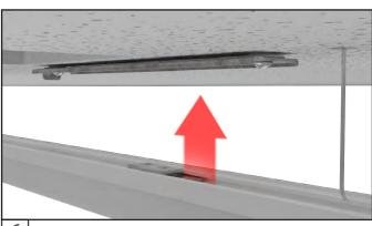
6 Raise fixture up to ceiling so that magnets are in line with magnetic attachment plate
