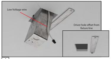
Cut 4x3" for 25W driver box hole in ceiling where the end of the fixture with electrical connector will be. Connect driver box to power source and insert into ceiling. Leave low voltage wire accesible from room side.
