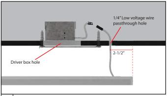
Drill 1/4" hole 2-1/2" from end of fixture for low voltage wire passthrough. See shop drawings for location of safety wire passthrough hole.
