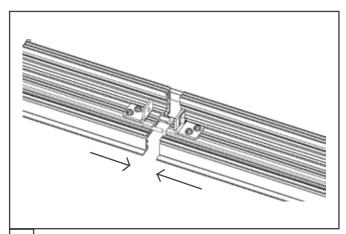
Align Guide pins and slide fixture sections together. Ensure that no wires are pinched.
