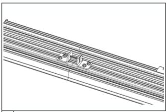
5 Insert joiner screw through male L bracket and thread into female L bracket.
