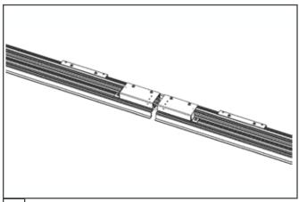
1 Secure fixture sections to grid, ensure hook is attached over the TBar.
