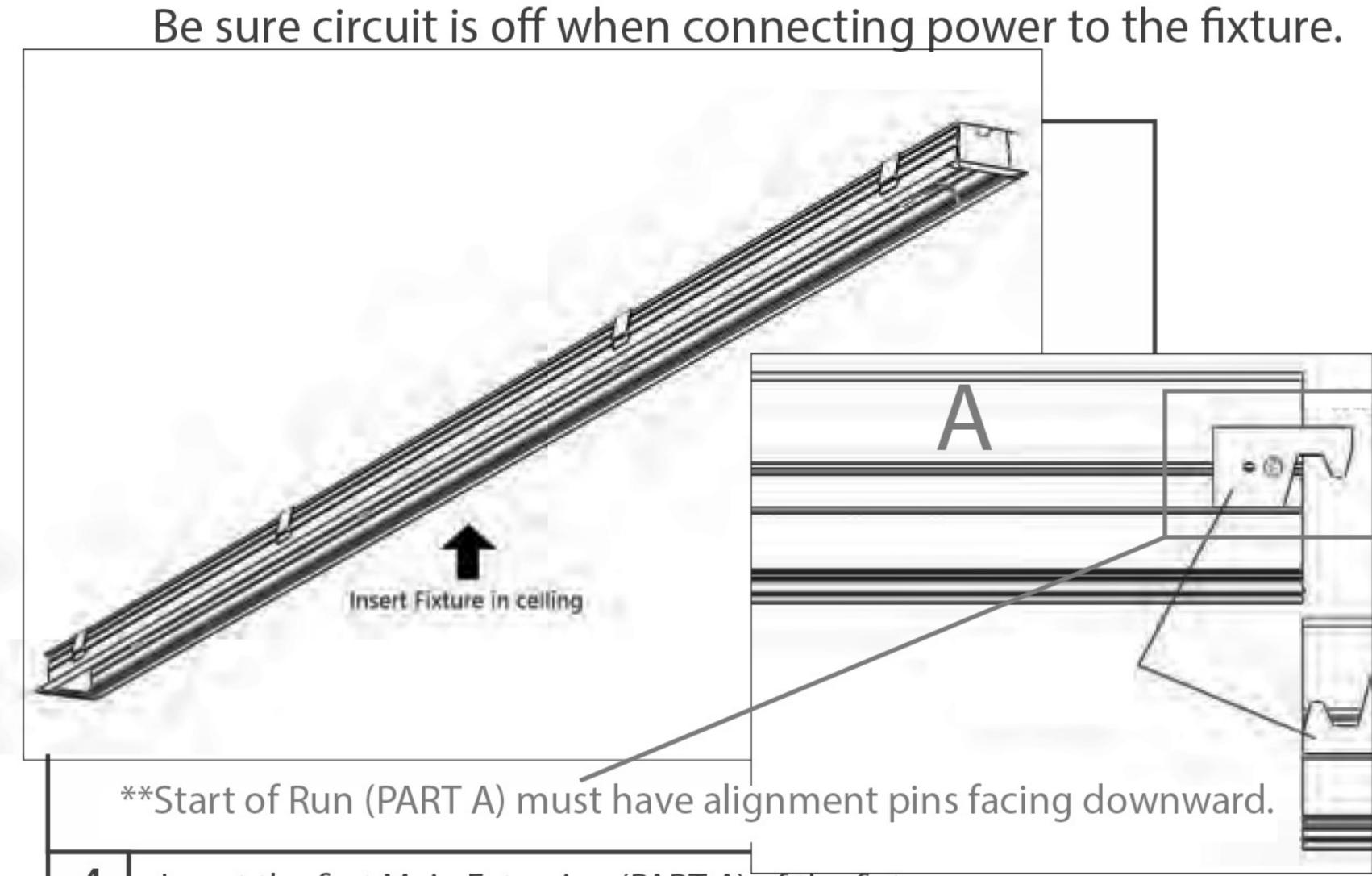
Insert the first Main Extrusion (PART A) of the fixture run into the cut hole. See shop drawings and fixture labels for location within run. PART A MUST Be installed first to ensure proper alignment of pins (See diagram above).
