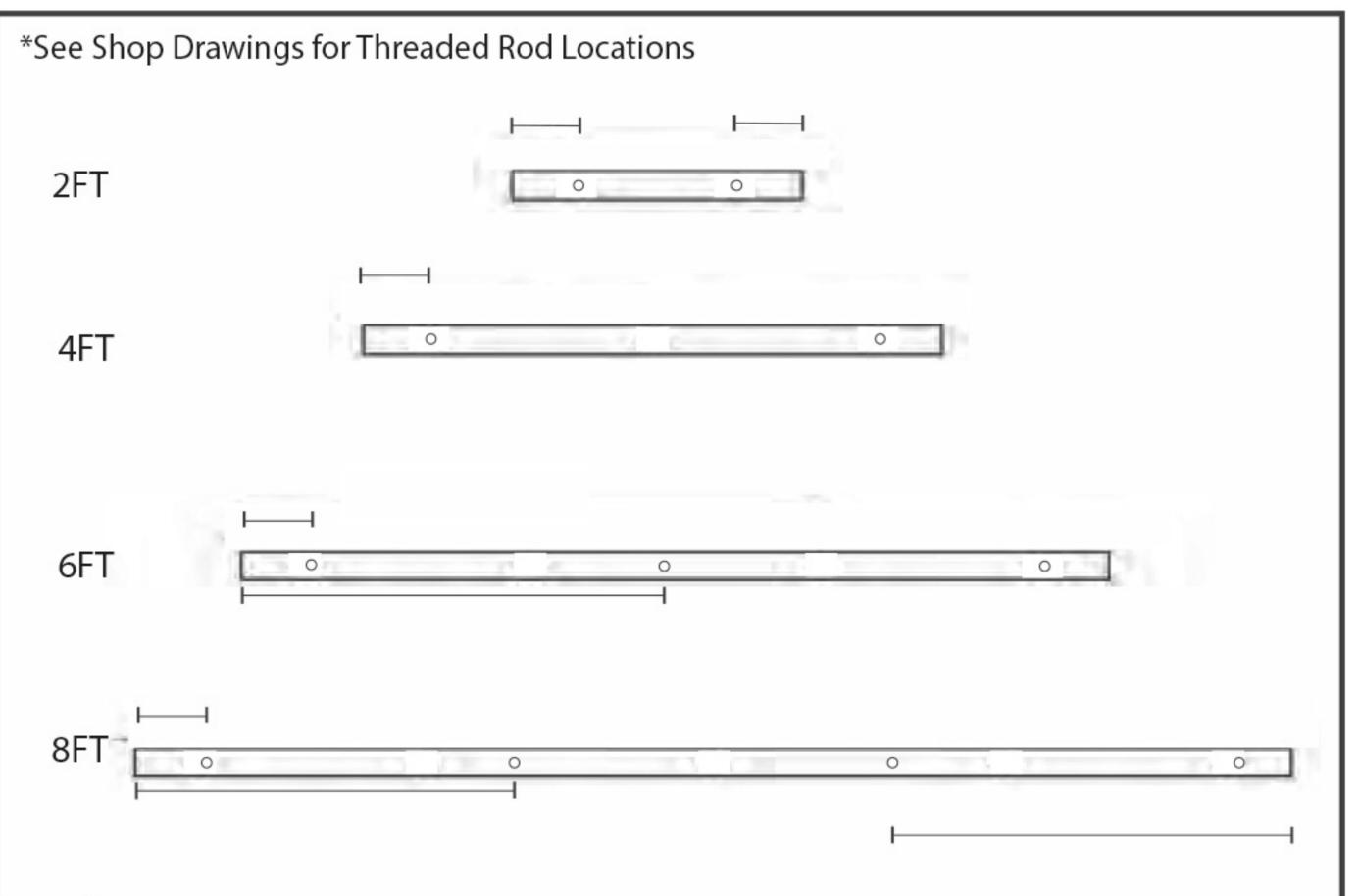
If using 1/4-20 threaded rod installed from structure, see location holes in shop drawings provided.
