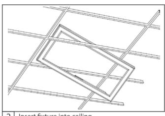
2 Insert fixture into ceiling
