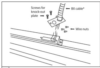
6 Remove access plate and attach appropriate wires. Ensure connections comply with local and national codes.
