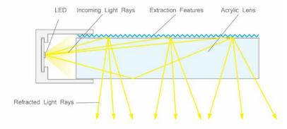
**Edge lighting** is a method of optical tranmission that Aron uses in many of our fixtures. Light coming from the LED shines into an acrylic lens. On the top side of the acrylic, surface bonded extraction features help to refract and spread light rays out of the arcylic to create various beam shapes.
