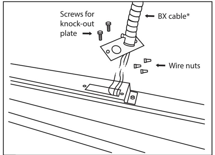
6 Remove access plate and install BX connector through the knock-out. Connect wires from the BX cable to wires on driver using wire nuts. If dimmer is required, connect appropriate wires to grey/purple wires on the driver. Ensures connections comply with local and national codes.
