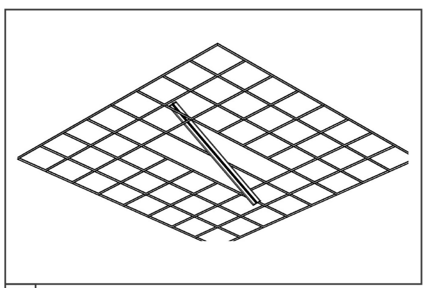
Insert fixtures into ceiling grid - parts are labeled (A, B, C) for location in the continuous run.
