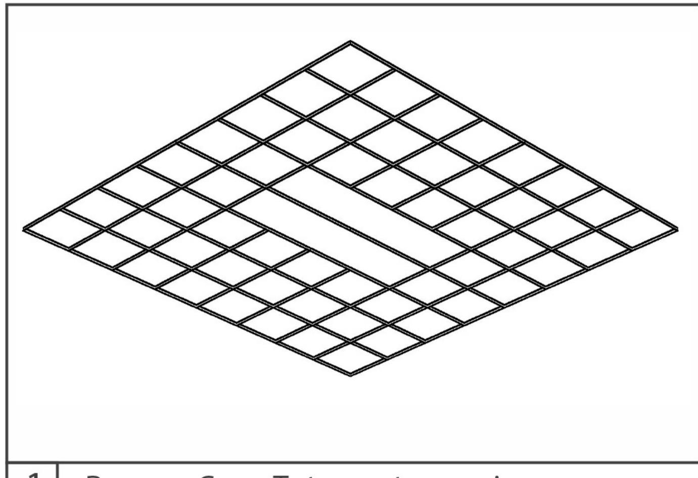
Remove Cross-Ts to create opening for fixture run.
