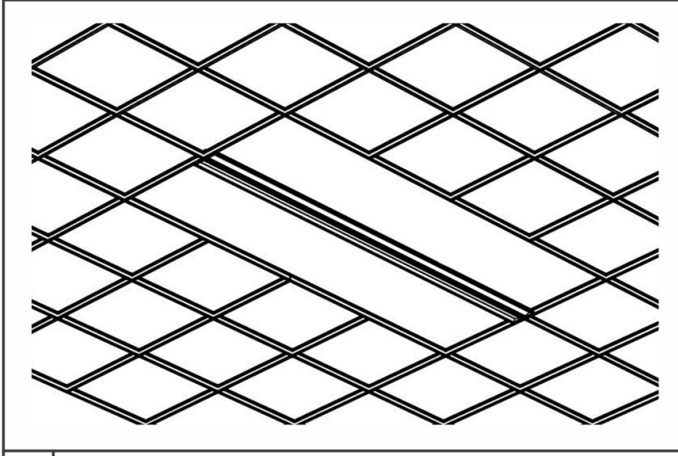
3 Lay fixture onto center T-Bar.
