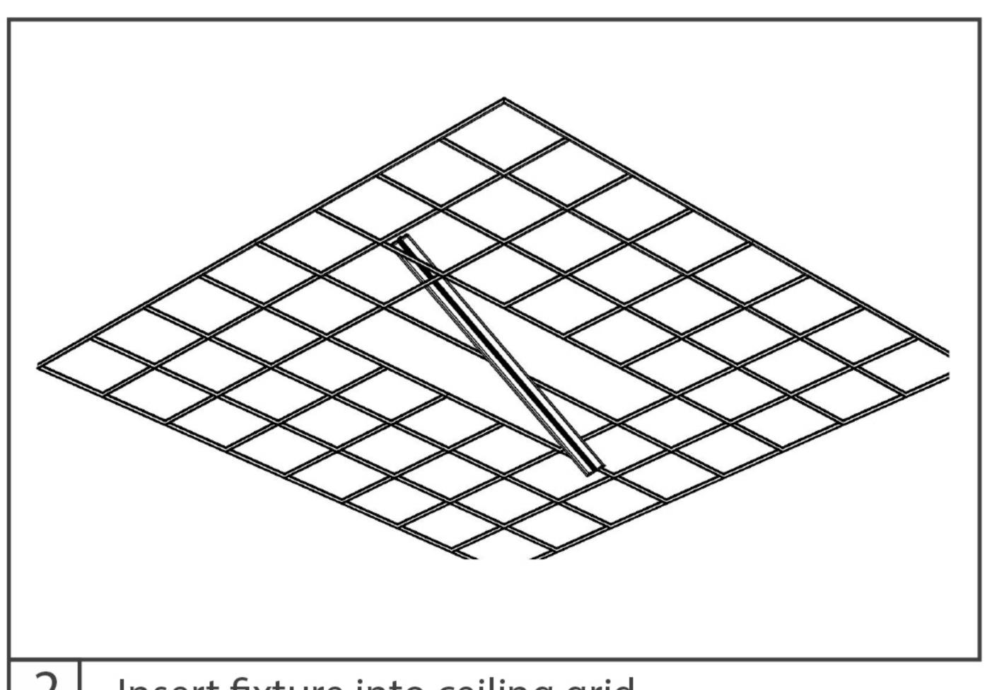
2 Insert fixture into ceiling grid.
