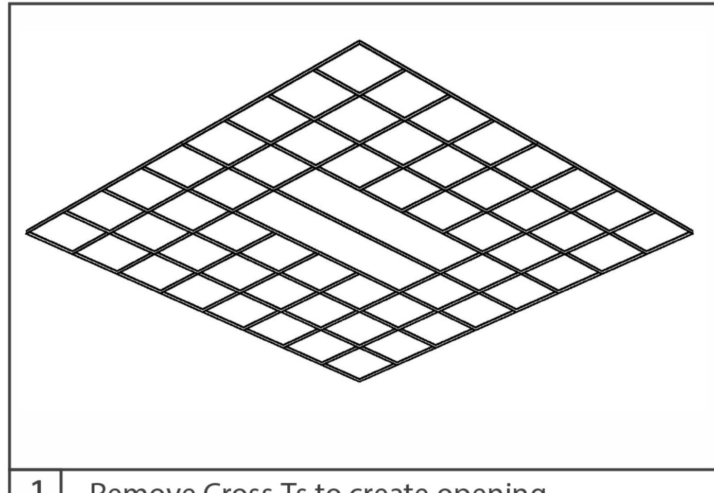
Remove Cross-Ts to create opening for fixture.
