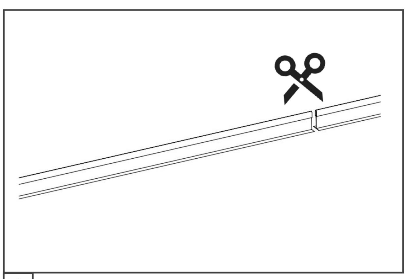
Cut T-Bar to lay on flange of fixture.
