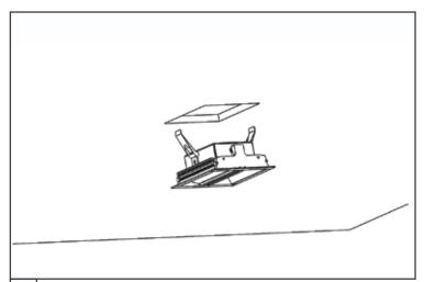
Bend both springs upward at the same time and install the fixture into the ceiling
