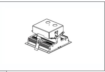
2 Complete all electrical wiring with the fixture still below the ceiling. Remove the top cover to access wiring by removing 4 screws.
